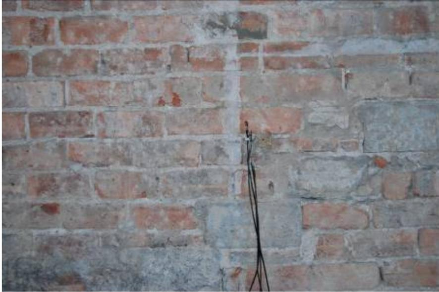
Fig. 8. Probes were set into the masonry to track any changes in humidity levels
