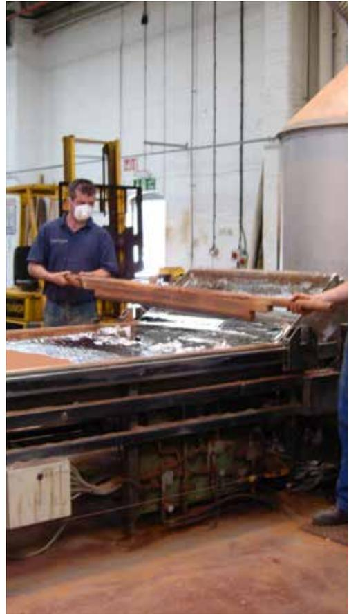
*Fig. 4* The manufacture of sand cast lead sheet.
