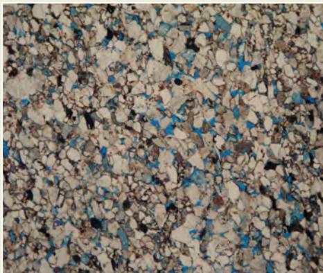
*Fig. 3-4: Studying sandstones under the microscope can reveal significant differences in stone structure. The images show red sandstones from different quarries, which appear visually similar, but have very different physical properties.*
