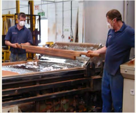
*Fig. 4: The manufacture of sand cast lead sheet.*
