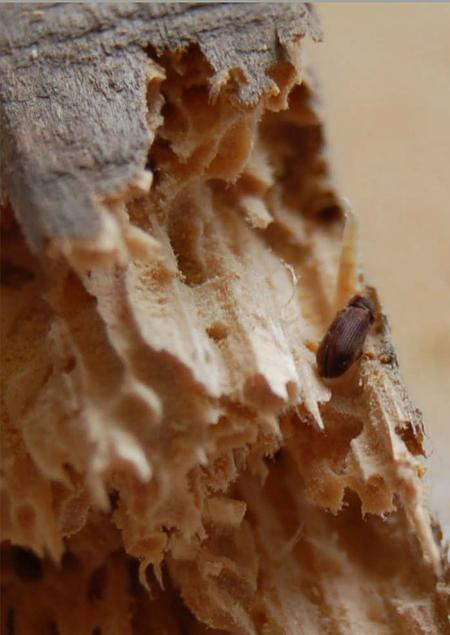
*Fig 1: Wood damaged by furniture beetle*
