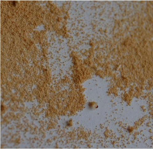
*Fig. 2: Bore dust of the common furniture beetle*
