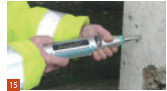
Fig. 15 Elastic surface rebound hammer (Schmidt hammer) Chris Wood © English Heritage.
