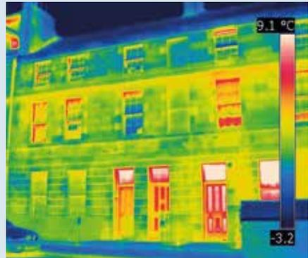
*Fig. 1 Thermal imaging of an elevation. The windows on the bottom left have the shutters closed and are showing a reduced heat loss compared to the open shutters above.*
