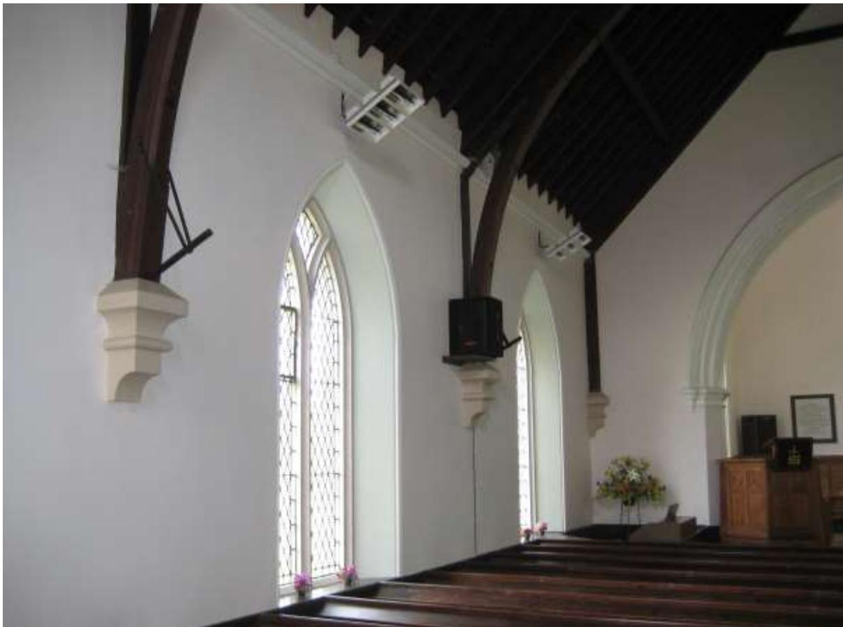
Fig. 3: *Hobkirk Church in the Scottish Borders is heated by radiant panels at cornice level*
